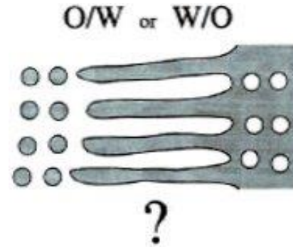
Fig. 9-7: Which type of emulsion forms depends on which type coalesces the faster.
