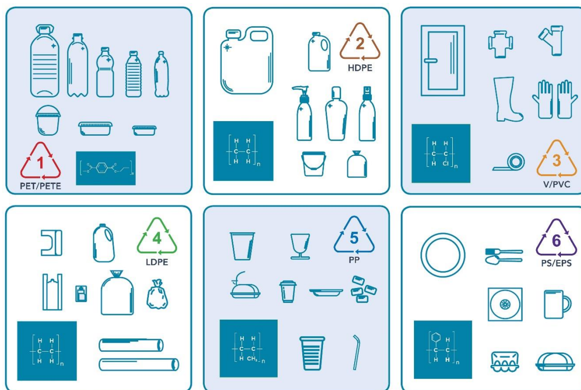
Figure 1. Examples of some common commodity plastics and their uses. The chemical structures of the constituent polymers and the corresponding recycling codes are shown. Adapted from reference 3 .
